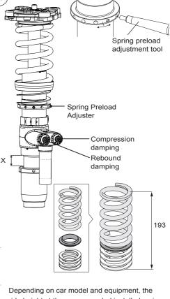
Depending on car model and equipment, the ride height at the recommended installed spring package length may vary.
